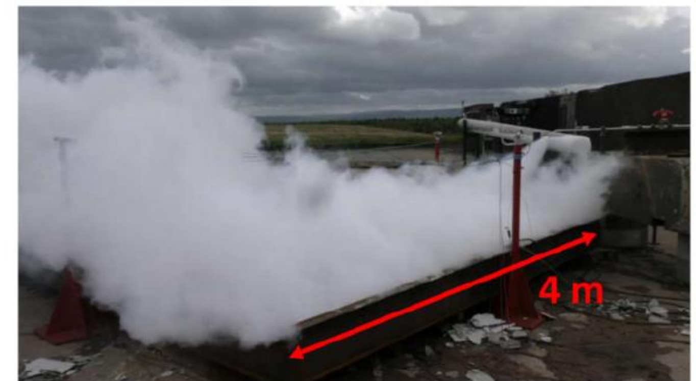
Figure 11: RS-3F refrigerated, pressurized ammonia release
